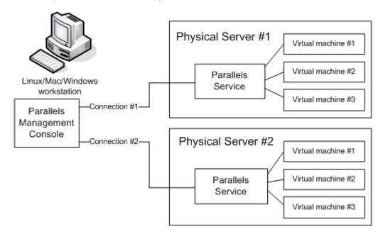
Parallels Management Console uses a typical client-server architecture.
